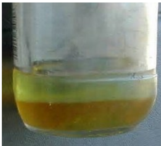
Diesel fuel sample showing water and sediment contamination.
